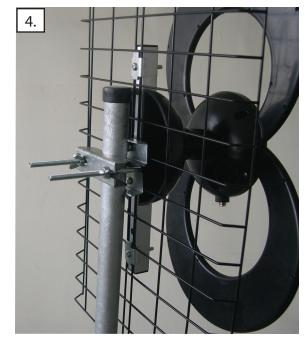
**4. Assembly complete.** Attach the C2 antenna to any kind of mast or mount (up to 2" in diameter) with the adjustable U bolt clamp. The 75 ohm coax connector is in the center front.
