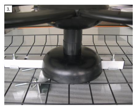
**3.** Align the two halves of the separating column and attach the reflector (grid) to the antenna elements (Tapered loops) by threading the bolt through the center of the column. Tighten.
